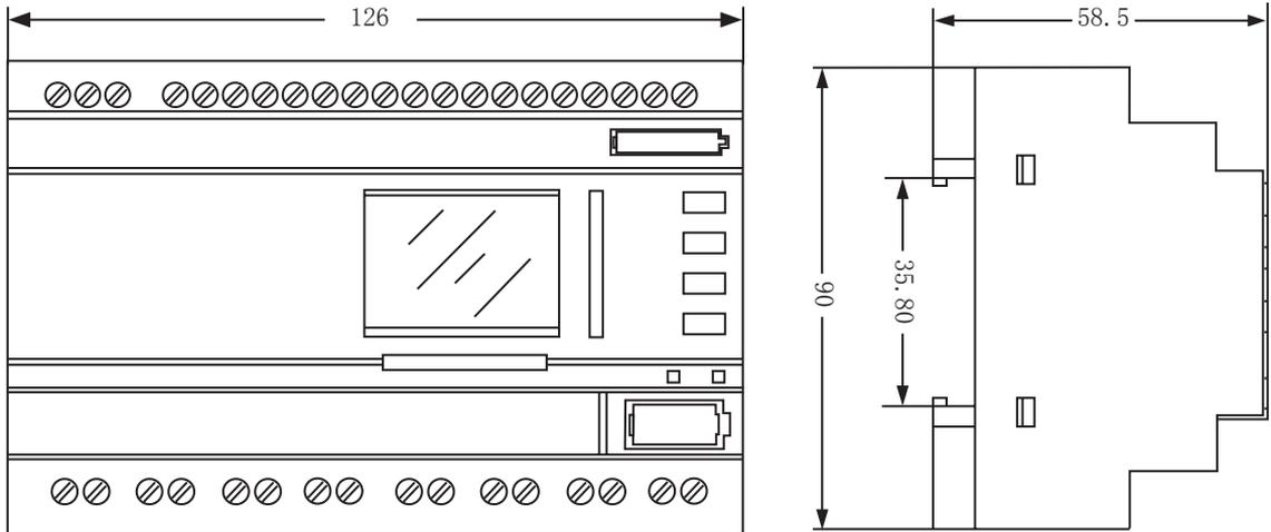
Installation Dimension of APB-22 Series (mm)
