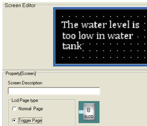
Connect the analog comparator block B0002 to SLCD. When  $P1 < 1V$ , the analog comparator will output signal and the alarm message will be displayed on PLC display screen.
