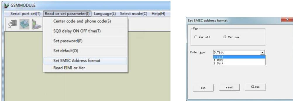
SMS Module information transmission coding format is selected for three types: 7bit, 8bit and USC2, USC2 is the factory default format. When SMS module only receive not send and the factory default format is USC2, customer can choose the other two coding format to use the SMS module.
