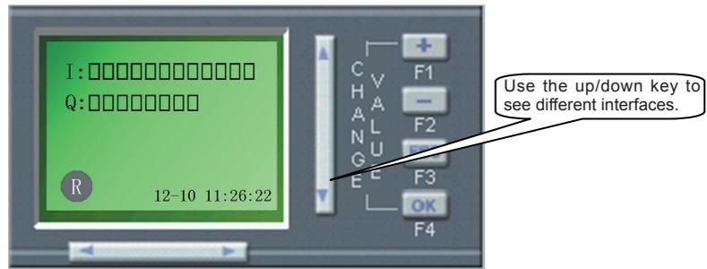
The current value and parameter of various timer, counter, and analog comparator can be displayed on APB-HMI. There are two data displayed on this HMI: Current value and Parameter value. The interface can be modified, added, and deleted according to your needs.
