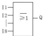
In NOR function block, when the status of all inputs is low potential (status 0), the output is connected (status 1). If any one of the input is high potential (status 1), the output is opened (status 0).
