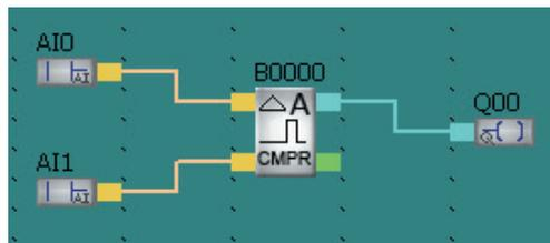
Input 1 is connected to AI0
