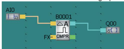
Input 1 is connected to AI0;
