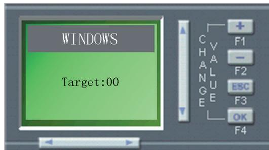
On this interface, press “OK” key to modify the target number that needs to be jumped to.
