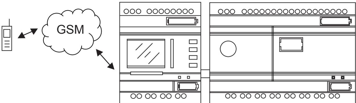
When SMS works in mode 0 APB PLC input state can be inquired and output state. time and count parameter.
