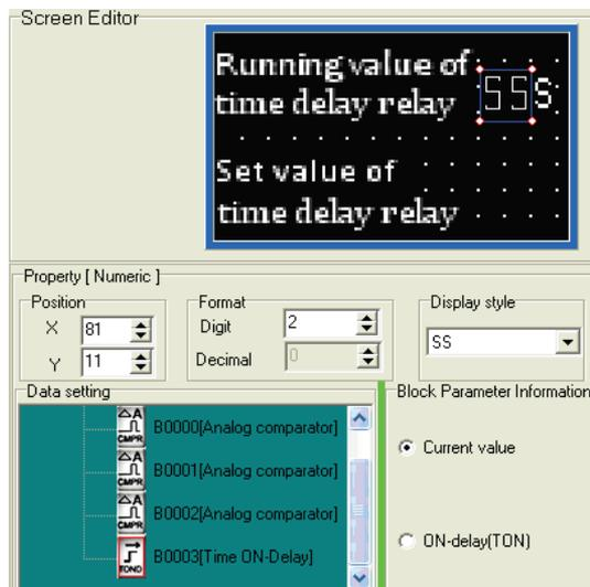
Choose the component “B8”, and select “Function block B0003 (on-delay). The “ON-delay” is chosen as the parameter. Displayed digits: 2; decimal digits: 0.
