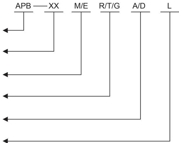
Note: M means main machine, E means extension module; R means relay output, T means NPN transistor output, G means PNP transistor output; A means AC type, D means DC type; C means real-time clock; The economical type is supplied without LCD panel, and the basic type is supplied with LCD panel.
