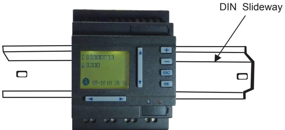
Use standard DIN rail for installation of APB
