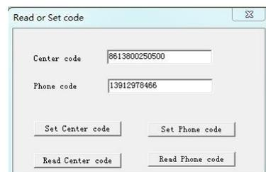
Input SMS center number and SMS mobile number. SMS center number is 20bits at most. It is the operating agencies message service center number of SIM card in SMS module, e.g.: 861380025500. "SMS mobile number": 20 bits at most. If it is not set, no any message will be sent when there is the alarm.
