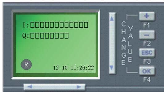
On this interface, it is able to observe PLC I/O status, and in the meantime, the current system time and PLC running status are displayed. Press “↑ ↓”key to jump to self-defined interface.
