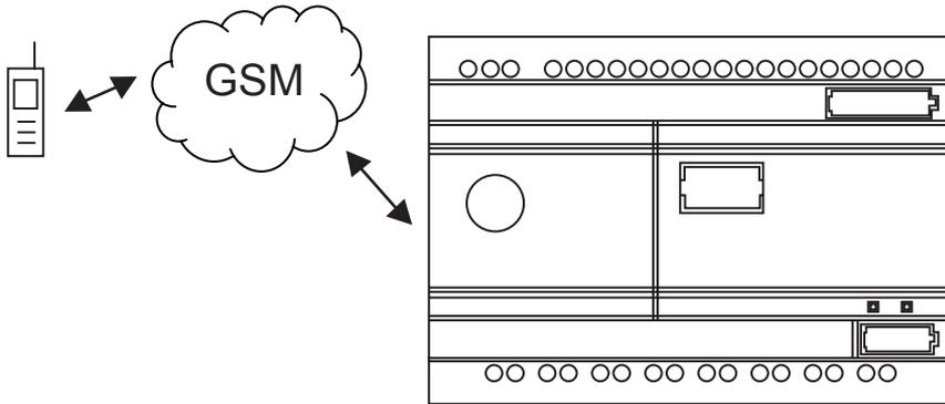
When SMS works in mode 0.Input signal SI1 has message alarming function. When the high level triggers SI1, the message“1ION”will be sent to the target number to alarm□The input and output state can be inquired and SQ1 can be set by sending the mobile phone instruction. Input signal SI0 controls the output SQ0 directly. The SQ0 delay ON OFF time can be set by GSMMODULE software.
