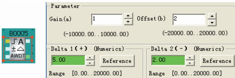
If the input value is 10V, then the theoretical value will be 12 according to the calculation formula: actual value =  $(Ax \cdot \text{gain value}) + \text{offset}$ , and the actual value is 12.01.
