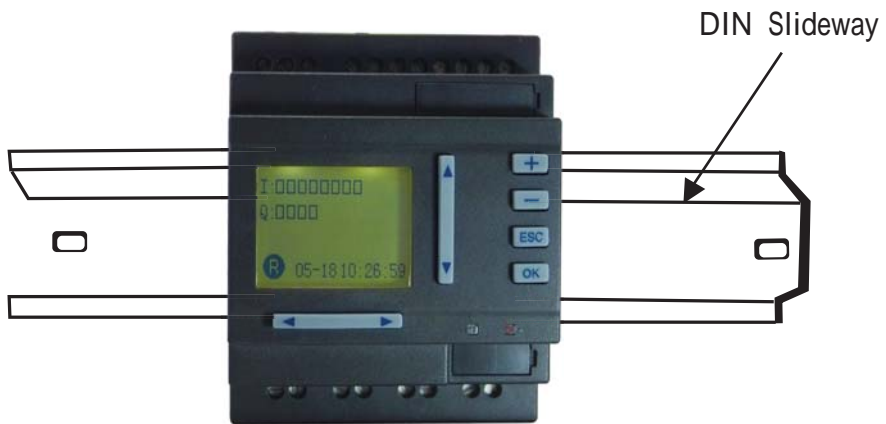
Use standard DIN rail for installation of APB
